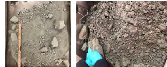
Figure 4. Sample of washed molasse (left) and wet molasse material (right) from Geneva Basin (Cern)
