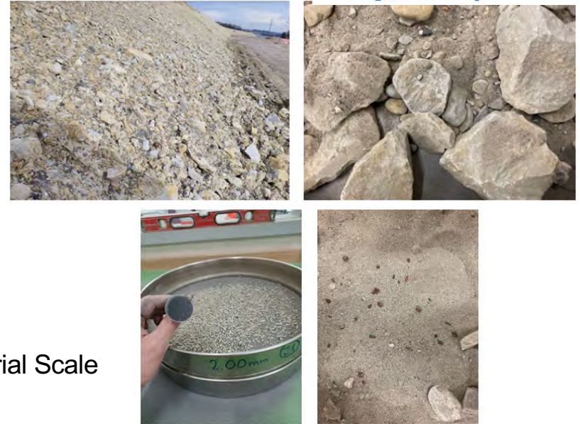
Figure 2. Sample of washed molasse from Gubrist Tunnel and iron residues
